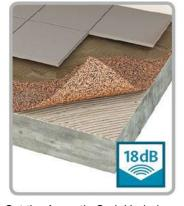
concrete slab. Always follow the glue manufacturers recommended instructions. Cut the Acoustic Cork Underlay to the desired length and install directly over the subfloor with crown of the rolled materials up, removing all trapped air. Butt the Acoustic Cork Underlay directly against the insulation perimeter barrier already installed. Put the loose laid material back. Using a properly sized
